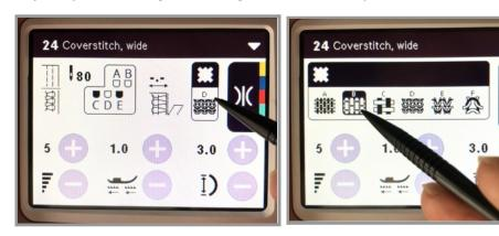
For stitches with a bold appearance on the fabric surface, use 12 weight cotton or topstitching thread in both needles - in place of regular overlock thread. When using thicker threads like these, be sure to use size 90/14 needles, which have a larger eye than the 80/12 needles, to accommodate the thread thickness. It is also recommended to increase stitch length.
